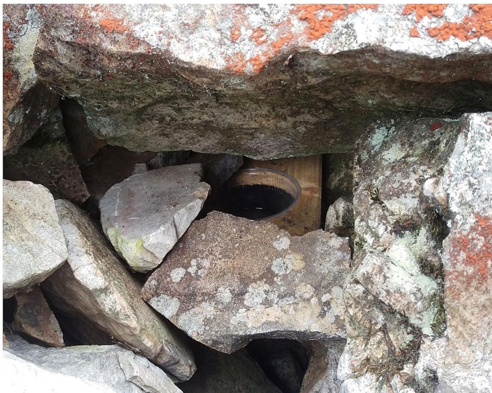
Fig. 2 Pitfall traps were placed in a holed wooden board and put deep in the gaps between rocks
